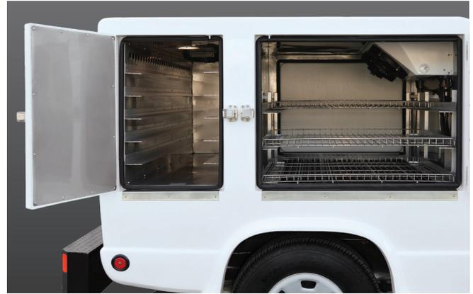
**The Body Series by Delivery Concepts** features lightweight, insulated fiberglass bodies with frozen, refrigerated, heated, and ambient compartment options, available in any combination. Models are available in 6-foot, 8-foot, and 11-foot lengths, making the Body Series a versatile temperature-controlled delivery solution for small businesses and large enterprises alike.
